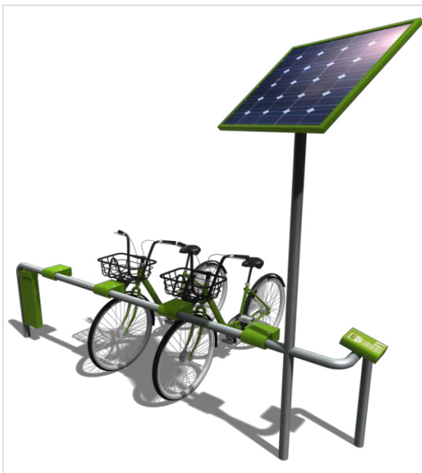
Figure 25 Conceptual layout of bicycle docking station with locking devices installed for individual bicycles with a solar panel for electricity generation
