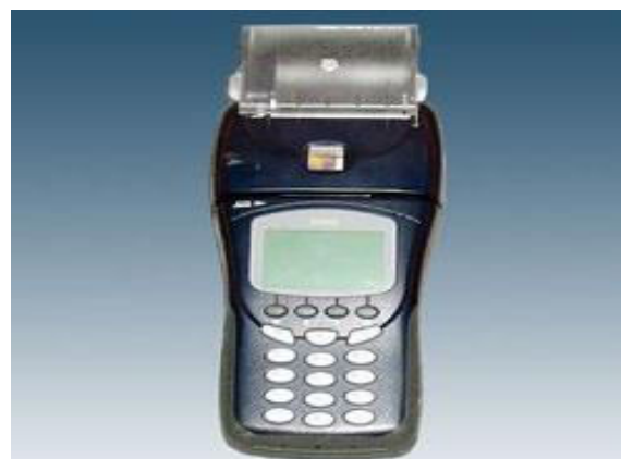
Figure 24 Typical handheld device used in the semi automatic system for fare calculation and issue of tickets
