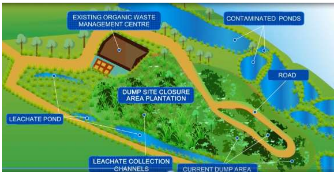
Dhapa Municipal Solid Waste (MSW) Dumpsite Green Capping, leachate Contamination Control & plantation development Restoration through bioengineering techniques Project under UK- aid under UK- KMC Low Carbon Resilient Kolkata by British Deputy High Commission, Kolkata Municipal Corporation ( KMC)
