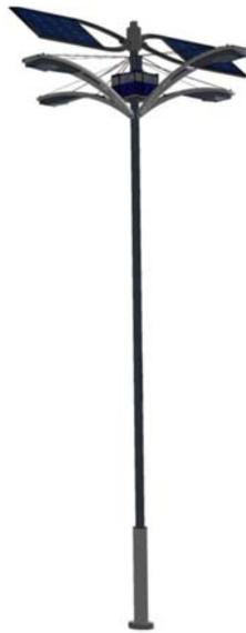
A Solar PV White- LED Street Light Double Arm consist of white LED luminary of 2\*12 Watt ( LED + Driver) as per configuration along with solar PV modules and LI-ION PHEROPHOSPHATE battery of given capacity, necessary control electronics-inter connecting wires / cables, module mounting structures etc. to operate the load for dusk to dawn. The broad performance specifications of a White Light Emitting Diode (W-LED) light source based solar street lighting system are given below:
