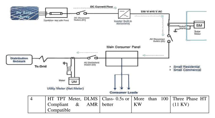
**Two Meter Configuration without Storage** The metering protocol for 'Grid connected rooftop solar PV system without storage' and location of solar meter and consumer meter shall be in accordance with the schematic below:-
