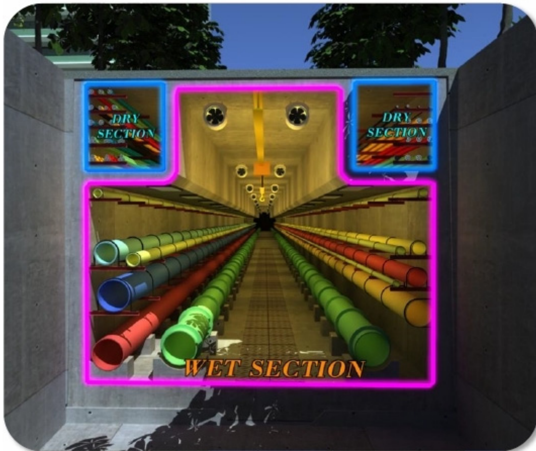
Figure 10 – Utility Tunnel, showing wet and dry sections [Source: Niles Puery b-2]
