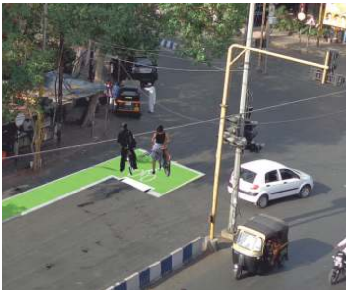
Identified waiting spaces for cyclists at junctions
