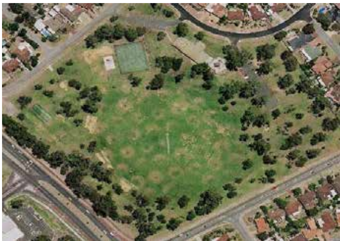
Example of poor Distribution Uniformity
