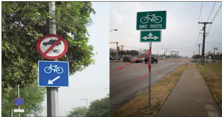
Figure 17.5: Signage's and markings on cycle track
