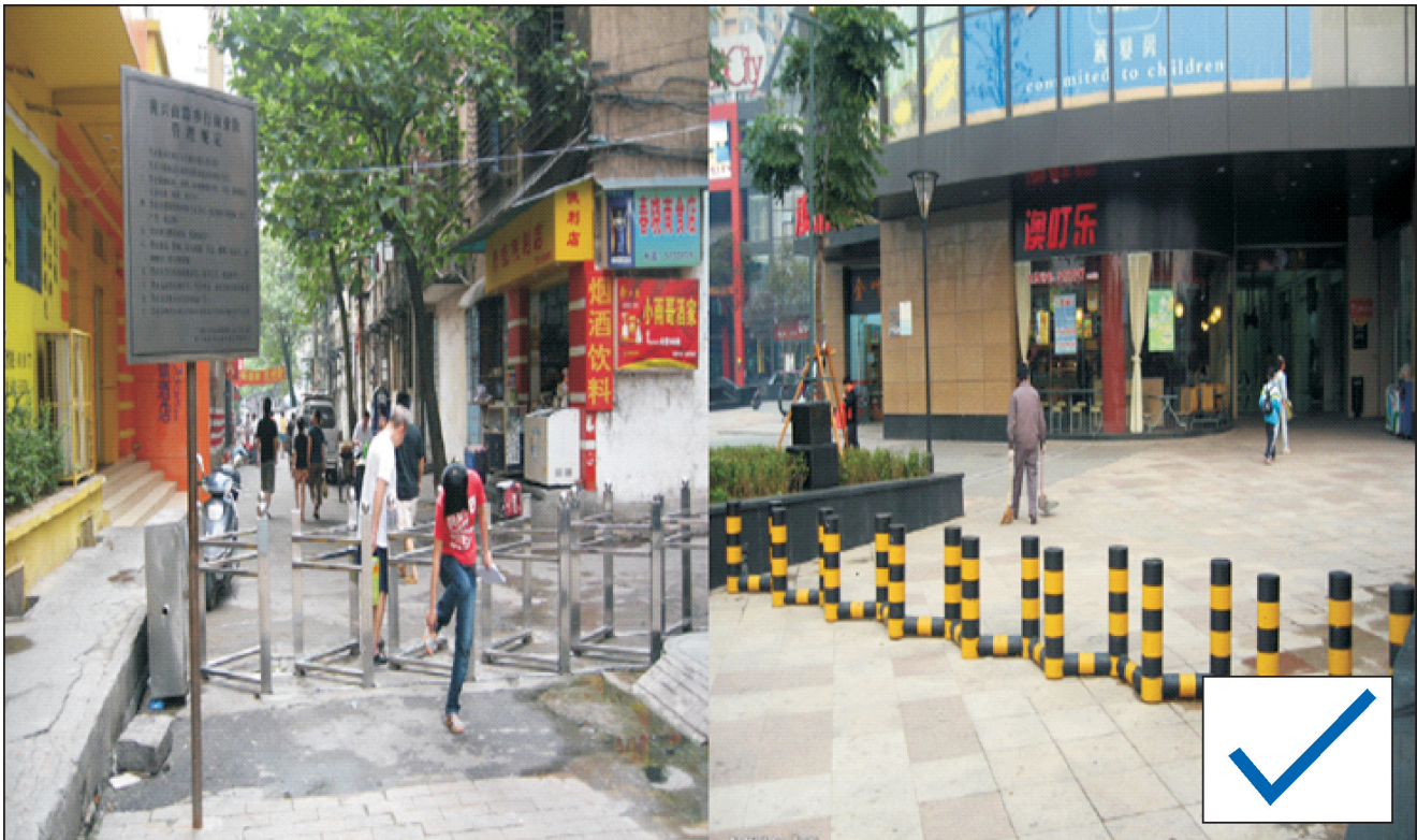
Figure 3.5: Designs to prevent encroachment
