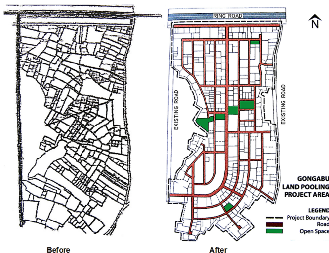
Figure 6: Plot division in Gongabu Land Pooling Project
