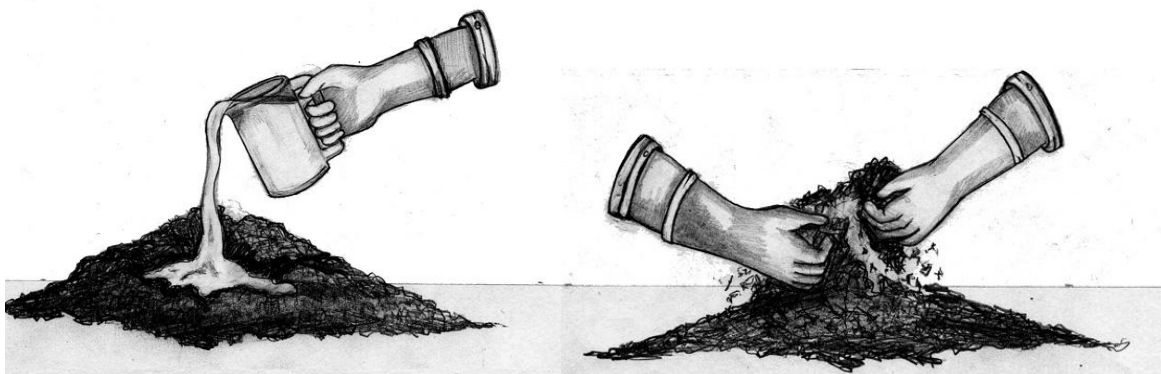
Figure 2-10: Make a mound of powdered char, scoop out a hollow and mix in the binder (like making bread).
