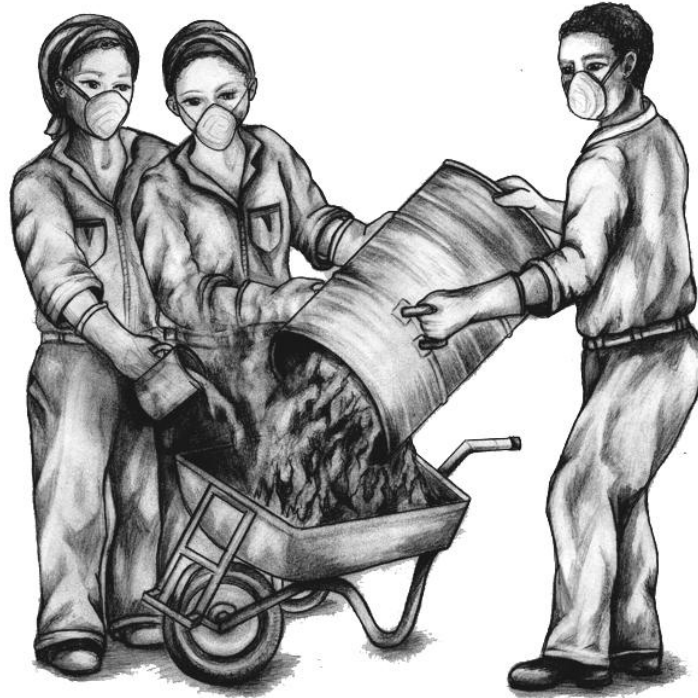
Figure 2-7: Tip the contents of the barrel into a wheelbarrow and sprinkle with water to stop it burning.
