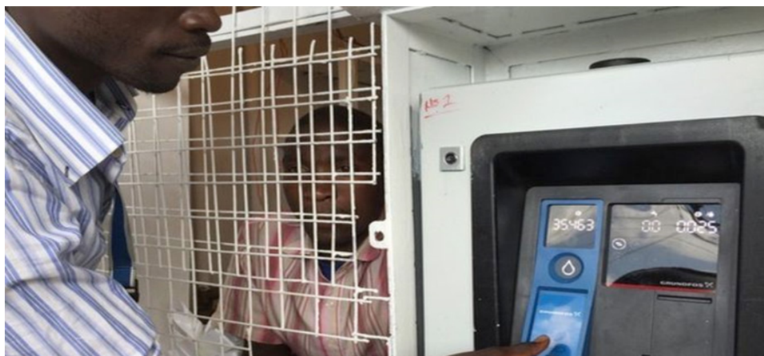
Figure 7: ATM water dispenser
