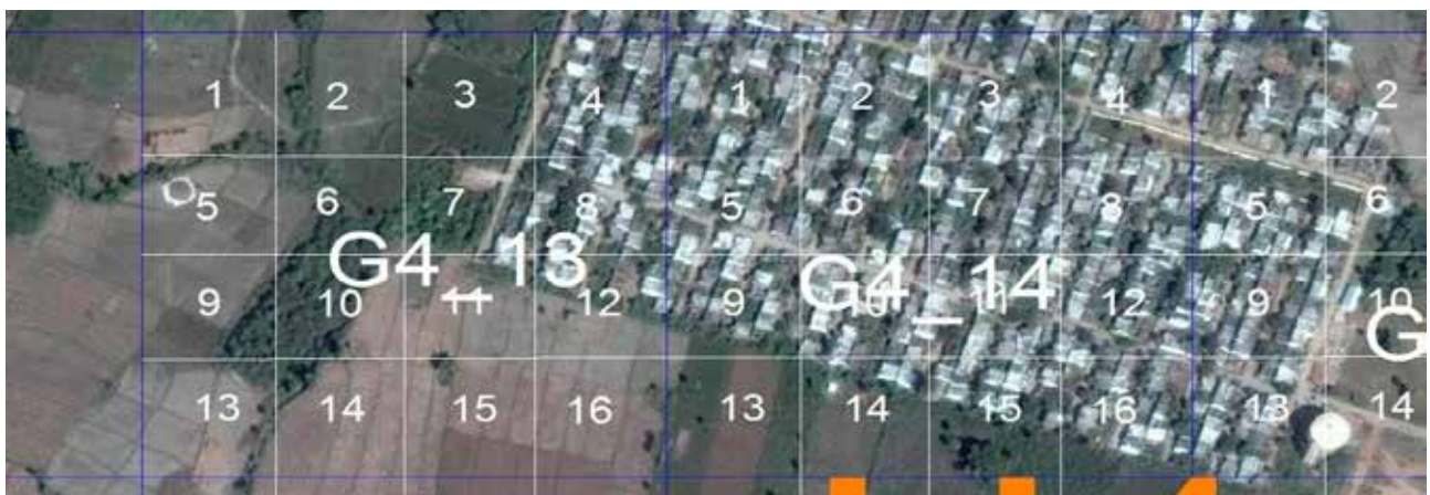
Grid of 250 m X 250 m size was demarcated on A1 size paper with 1: 500 Scale to map the features very accurately on ground
