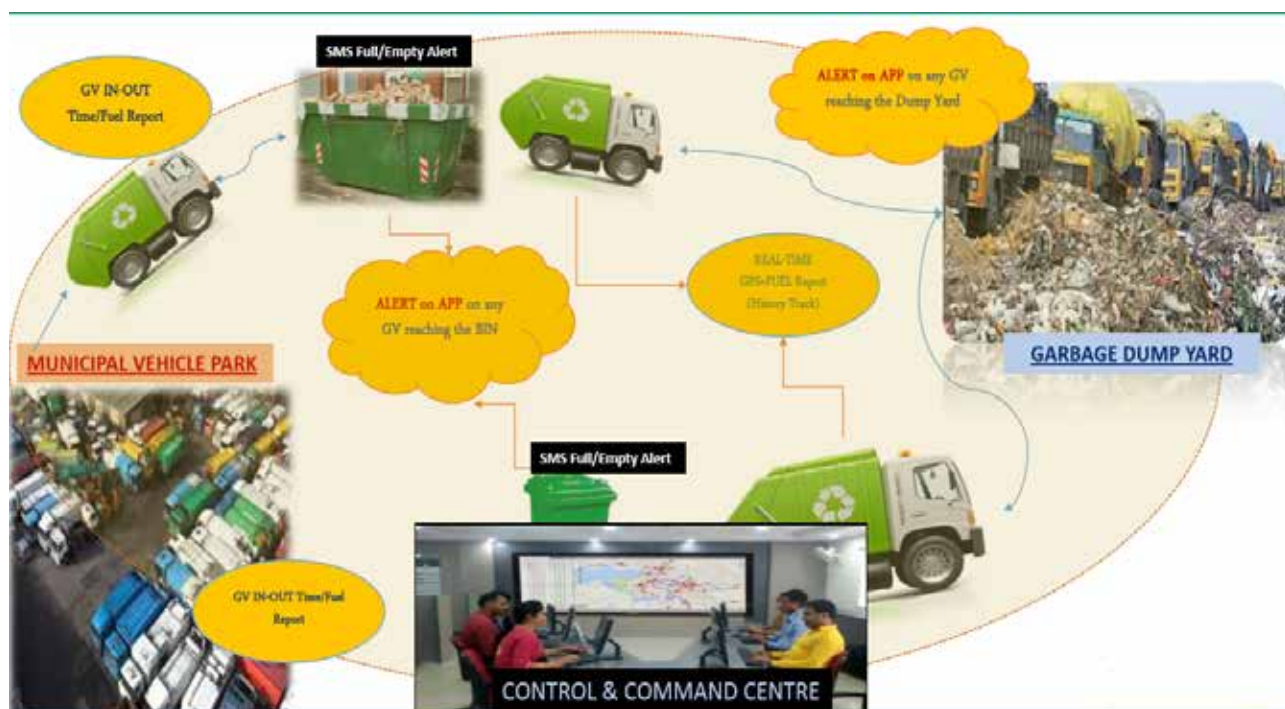
Functioning of RTVTS
