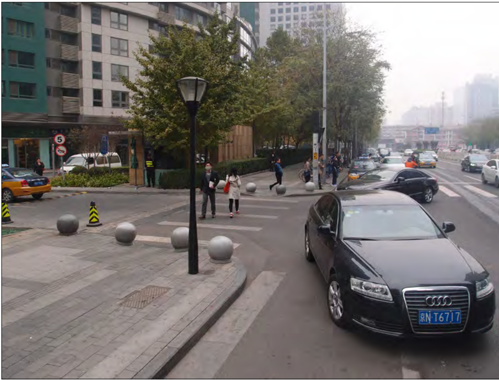
Existing driveway at the southeastern entrance of Xincheng Guoji prioritizes car traffic. Bollards are set too far apart leaving space for cars to park on the pedestrian crossing, blocking pedestrians. Illegal on-street parking is blocking the bike lane on Jintong donglu.
