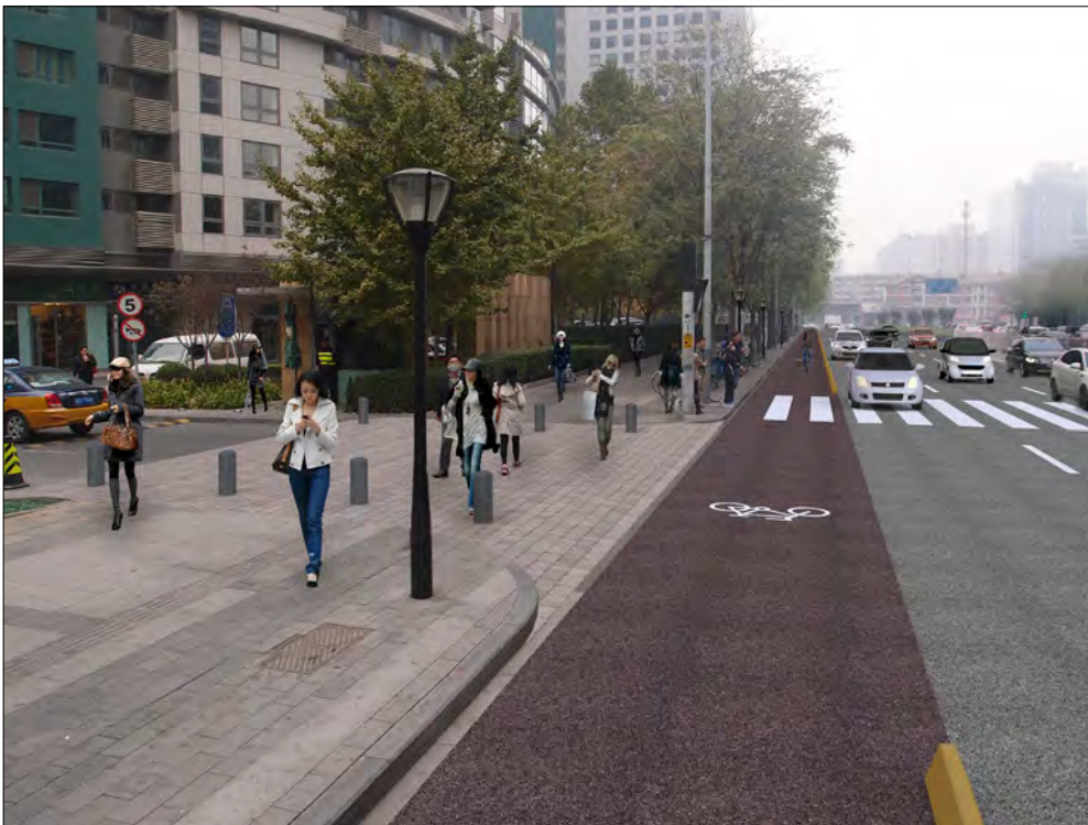
A raised, continuous walkway is proposed, where drivers need to slow down and give way to pedestrians. Bollards prevent illegal parking in the entrance and a curb is protecting the bike lane from illegal parking.
