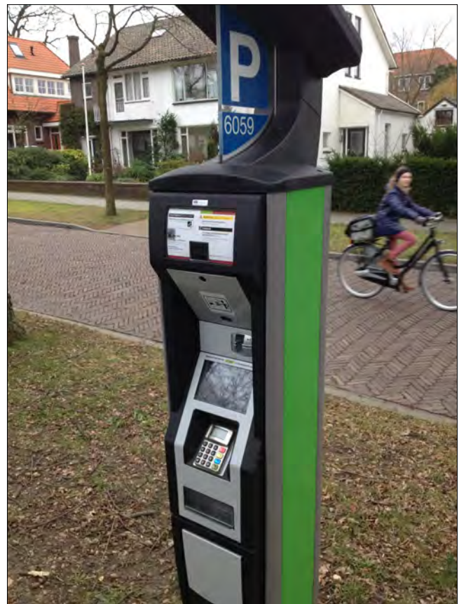
A solar powered parking meter in Nijmegen, the Netherlands. The number '6059' underneath the P sign represents the phone number for cell phone payment. After registering with the service online, drivers no longer need to use the parking meter and can pay through text messaging or with an app.
