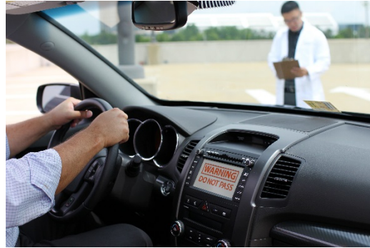
Figure 2-1: CV Application with do not pass warning on the vehicle dashboard (Source: USDOT)
