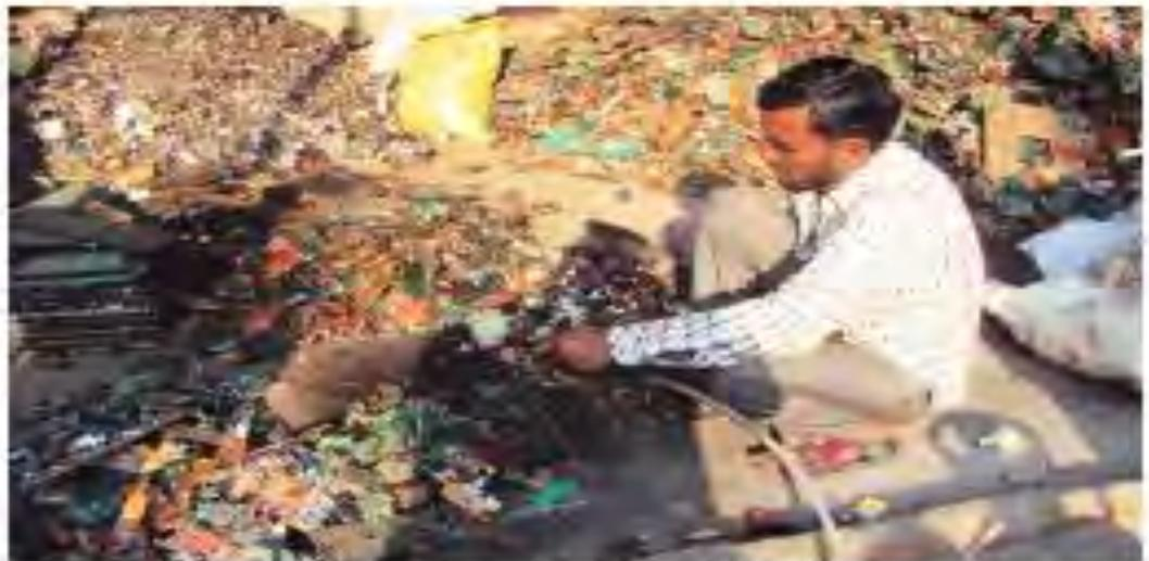
A worker using blow torch/flame to loosen the soldering of a PCB, Bhojpur
