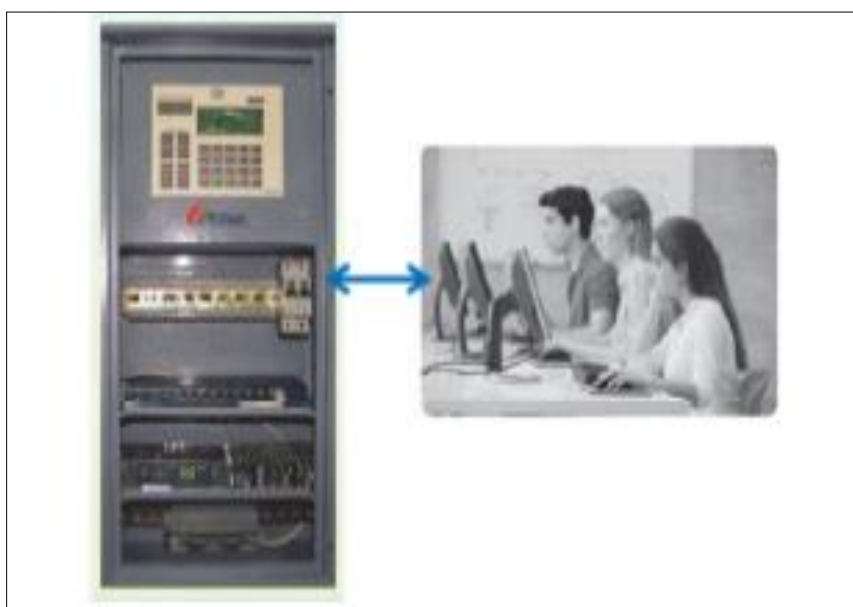
Figure 4-12: Fixed Time Controller with Control Room Connectivity Based Signalling
