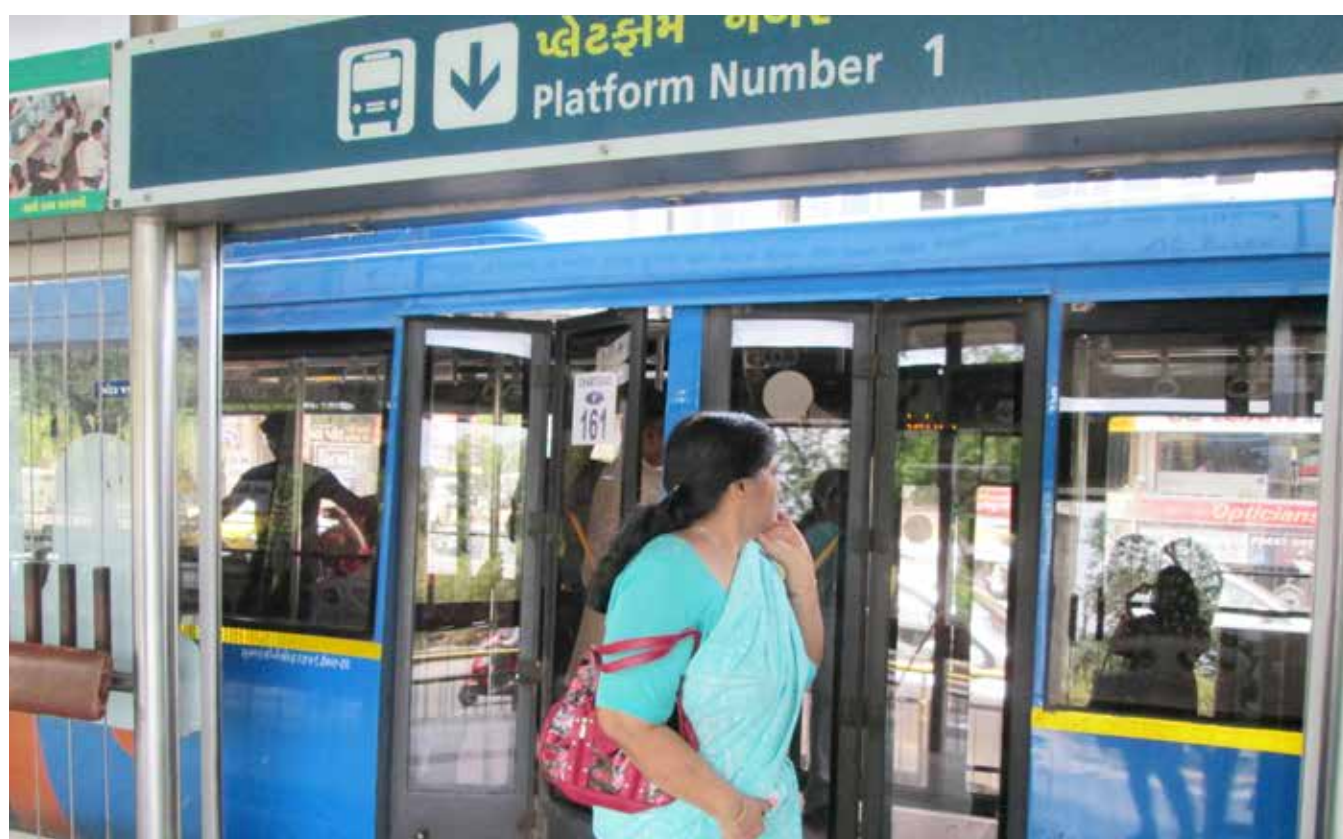
AHMEDABAD BRTS PROVIDES LEVEL BOARDING TO FACILITATE RIDERSHIP AND UNIVERSAL ACCESSIBILITY
