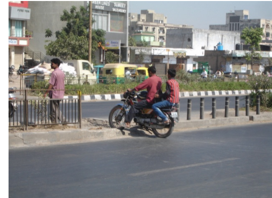
Picture 12: If adequate u-turn provisions are not made, smaller vehicles, like motorbikes, may resort to illegally using the pedestrian crossing to make u-turns.
