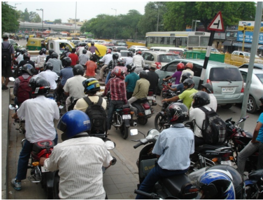
Picture 16: Poor intersection design, coupled with poor signal management, results in long queues on the mixed traffic lanes. This induced motorists to flout traffic rules, like waiting on the footpath, as shown in this picture.
