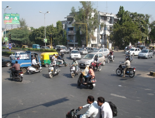
Picture 14: It can be very unsafe if the intersection of a minor street with the BRT is un-signalised, especially if vehicles are allowed to make a right turn across the BRT lanes.
