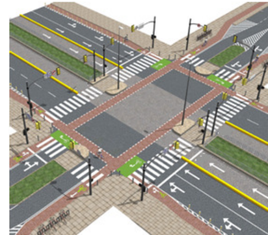
Picture 18: The Copenhagen turn is demonstrated here. NMT vehicles that want to make a right, continue straight into the intersection, and then position themselves in the green box in front of the intersecting road'
