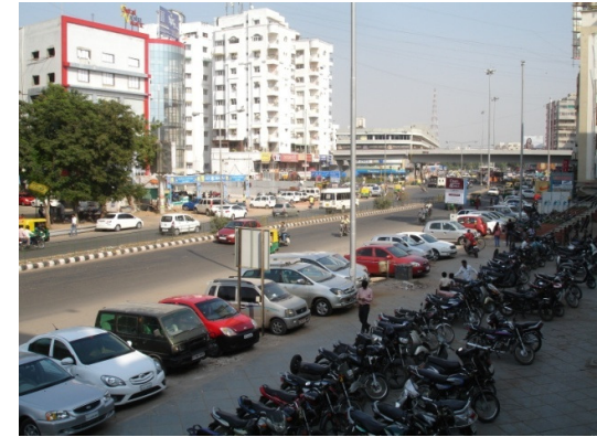
Picture 6: Urban arterials in most Indian cities are characterised by extensive edge development that have direct access from the main arterial. Such development generates local demand for parking, waiting areas, u-turns, right turns, pedestrian crossings, etc
