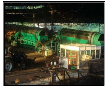
Fig: 4 Mechanical sieving in Level 1
