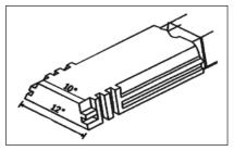
RCC channel roofing component
