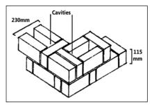
Figure 6: detail of rat trap bond
