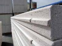
Interlocking edge of AAC wall panel
