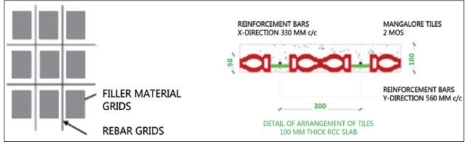
Detail of filler slab using Mangalore tiles.
