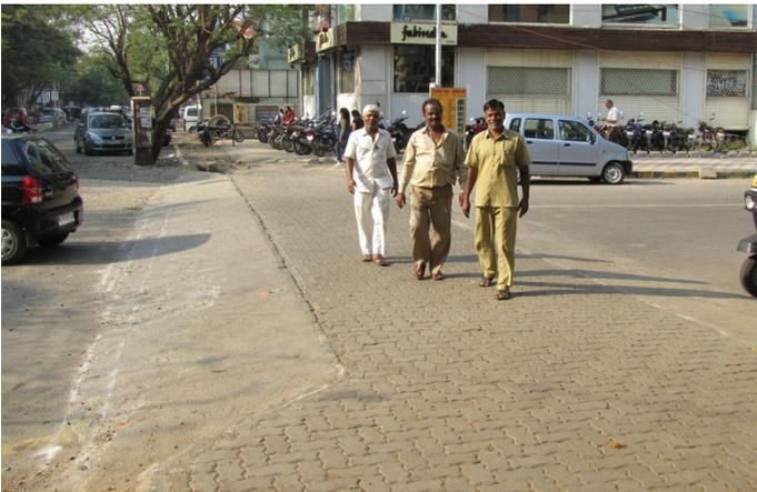
✓ Acceptable design for minor intersections. If the intersection is not signalised, it is acceptable to raise the crossings that are perpendicular to the minor arms while the crossing on the major arm is provided at grade.
