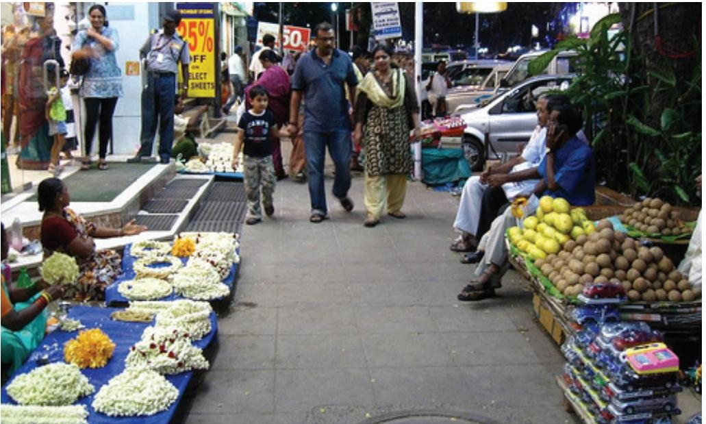
✓ Footpaths should be designed such that there is sufficient space for vending outside of the pedestrian zone (IRC:103-2012, 6.11.2).
