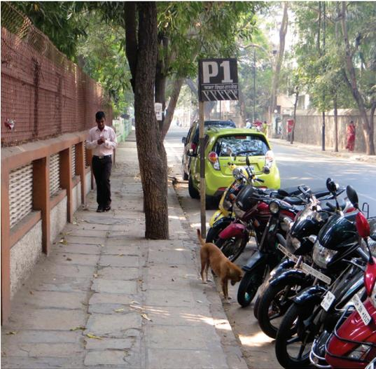
✓ Parallel parking for cars is preferred over angular or perpendicular parking because it saves space and is safer while exiting the parking bay. Parallel parking also doubles as perpendicular parking for cycles and two wheelers.
