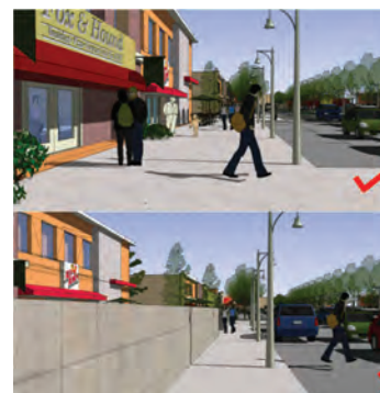
Figure 1.23: Remove compound wall and disallow front margin towards arterial streets
