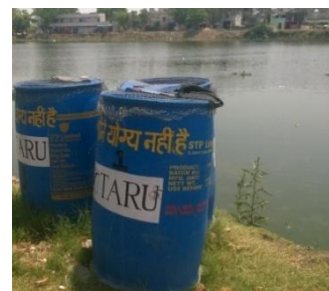
Picture 5: Experimental set up to chemically treat the lake water
