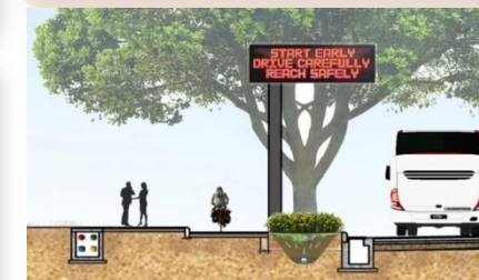
PROPOSED ROAD SECTION OF PB ROAD SHOWING UNDERGROUND UTILITY DUCTS
