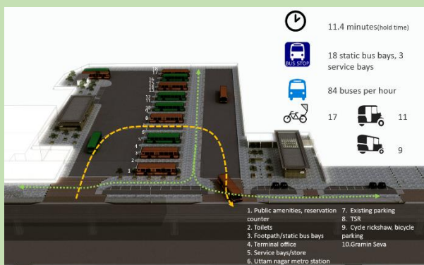
Figure 54: Area allocation & Bus circulation in terminal (Proposal 1)
