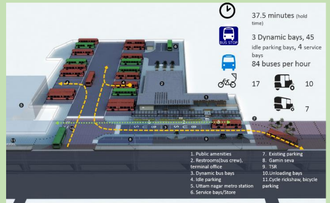
Figure 57: Area allocation & Bus circulation in terminal (Proposal 2)
