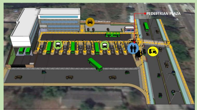
Figure 33: Pedestrian circulation in bus terminal
