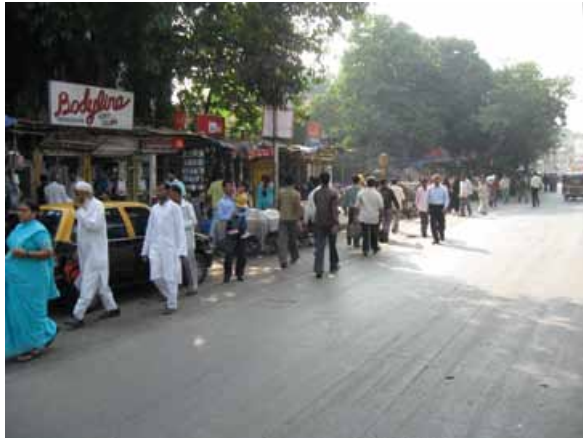
Figure 5.10 A pedestrian survey can identify locations where inadequate footpaths force pedestrians to walk in the street.
