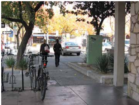
Figure 2.59 Utility boxes can be accommodated on easements at the edge of private properties, leaving the footpath free of obstructions.
