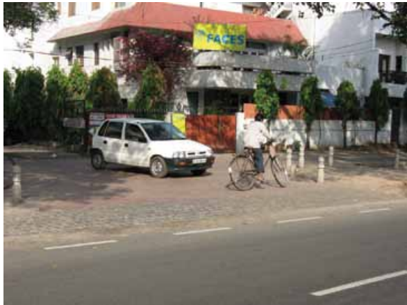
Figure 5.29 Similar to the intersection pictured above, the design proposes to raise the entrance to the small street by 150 mm so that motor vehicles slow down when they cross the footpath and cycle track.
