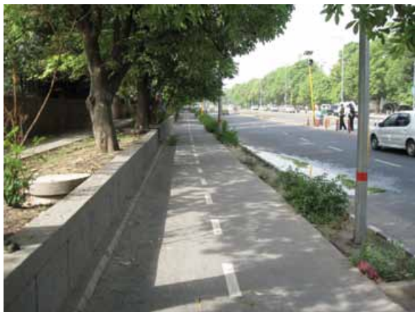
Figure 2.26 Tree lines should be arranged so that shade falls on footpaths and cycle tracks. Landscaping buffers can enhance the psychological separation between the carriageway and the cycle track or footpath.
