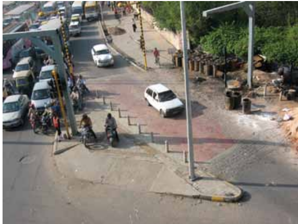
Figure 2.47 This left-turn pocket is raised and textured, helping to reduce car speeds and improving safety for cyclists who must merge with the left-turning cars if they wish to continue straight through the intersection.
