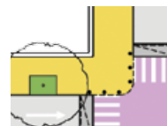
Figure 4.6 The boundaries of pedestrian spaces are defined by bollards to prevent encroachment by vehicles.
