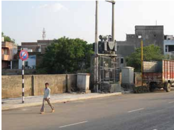
Figure 5.17 The street design should deviate from the standard section wherever there is an obstruction that is unlikely to be removed.
