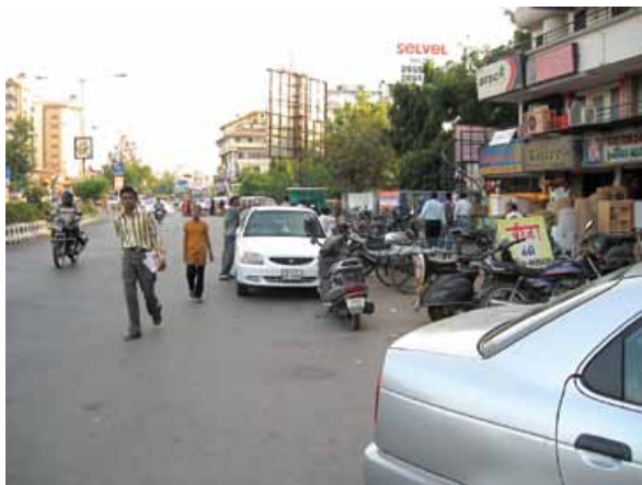
X Figure 2.40 When pedestrians encounter haphazardly parked vehicles, they generally walk next to moving vehicles because this part of the street offers the most direct route.
