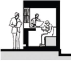
**A CONCRETE PLATFORM PLUS ROOF, WHICH DOUBLES AS A DISPLAY PLATFORM**
