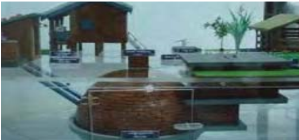
Standard model of the Farmer's Friend Biogas digester (Source: National Biogas Program)
