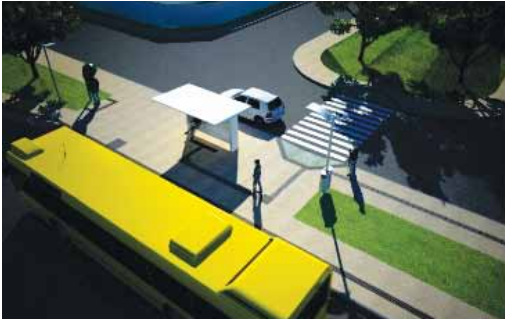
FIGURE 33: (A) BUS STOP AND PATHWAY SIGNALIZED WITH TACTILE DIRECTIONAL FLOOR: AS DESIGN AND BUILT SITUATIONS
