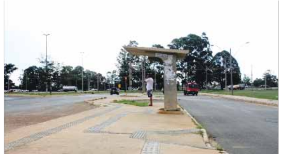
FIGURE 33: (A) BUS STOP AND PATHWAY SIGNALIZED WITH TACTILE DIRECTIONAL FLOOR: AS DESIGN AND BUILT SITUATIONS
