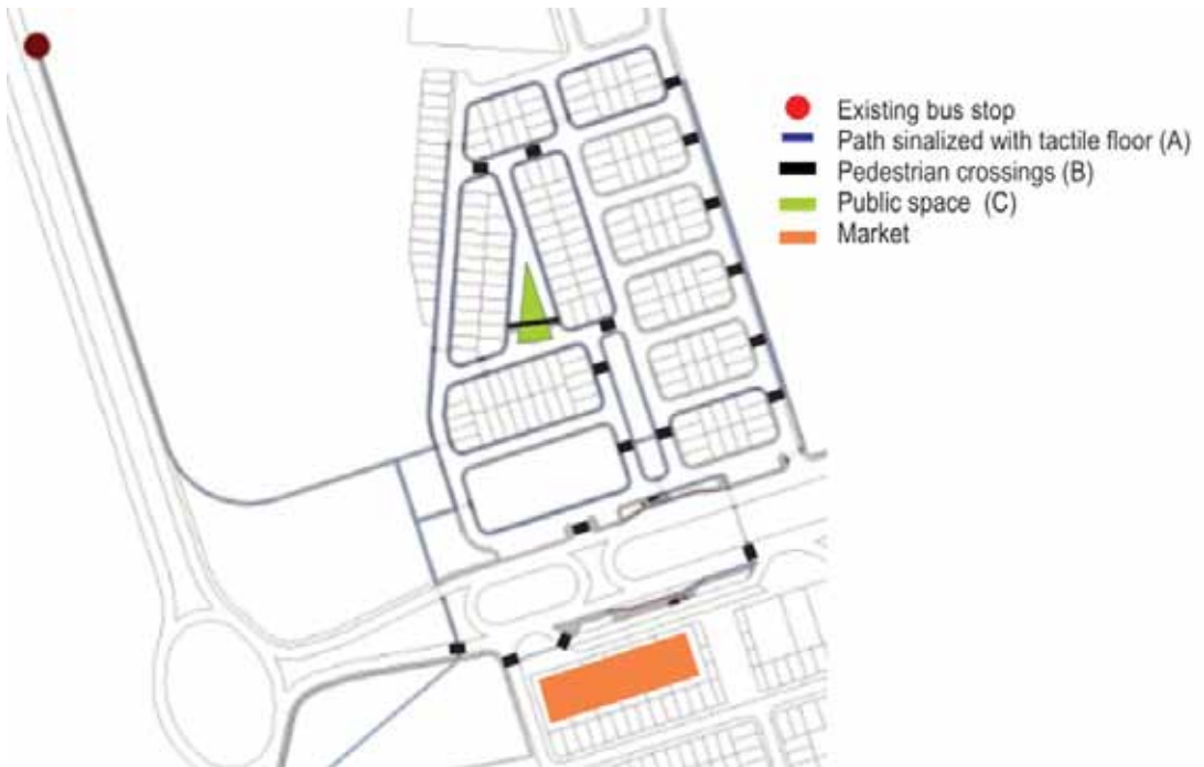
FIGURE 32: PEDESTRIAN FLOWS AND ACCESSIBLE ROUTES
