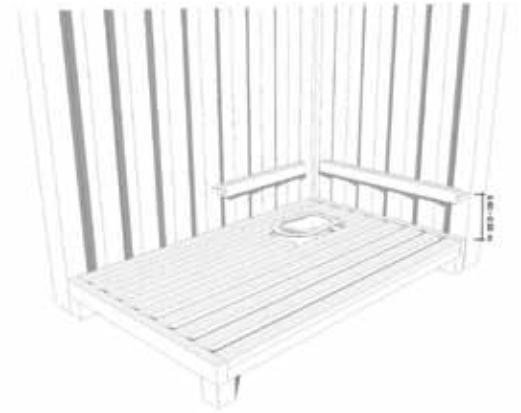
FIGURE 29: DRY FLAT TOILETS ON ELEVATED WOODEN FLOOR
