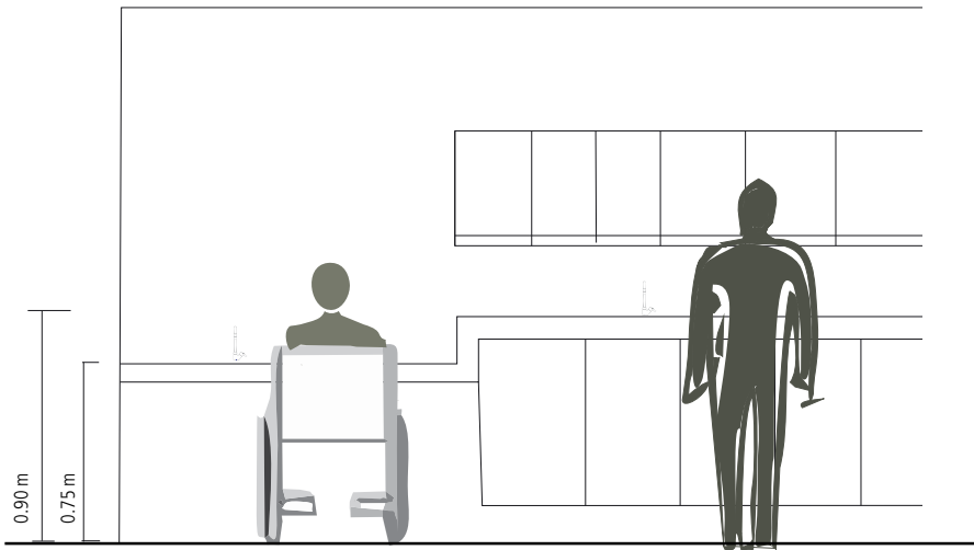
FIGURE 24: WORKING SURFACES, E.G. KITCHEN SINK
