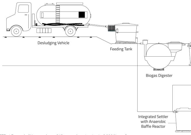
The FSTP at Devanahalli is spread over 615sqm and can treat upto 6,000 litres of faecal sludge a day.
