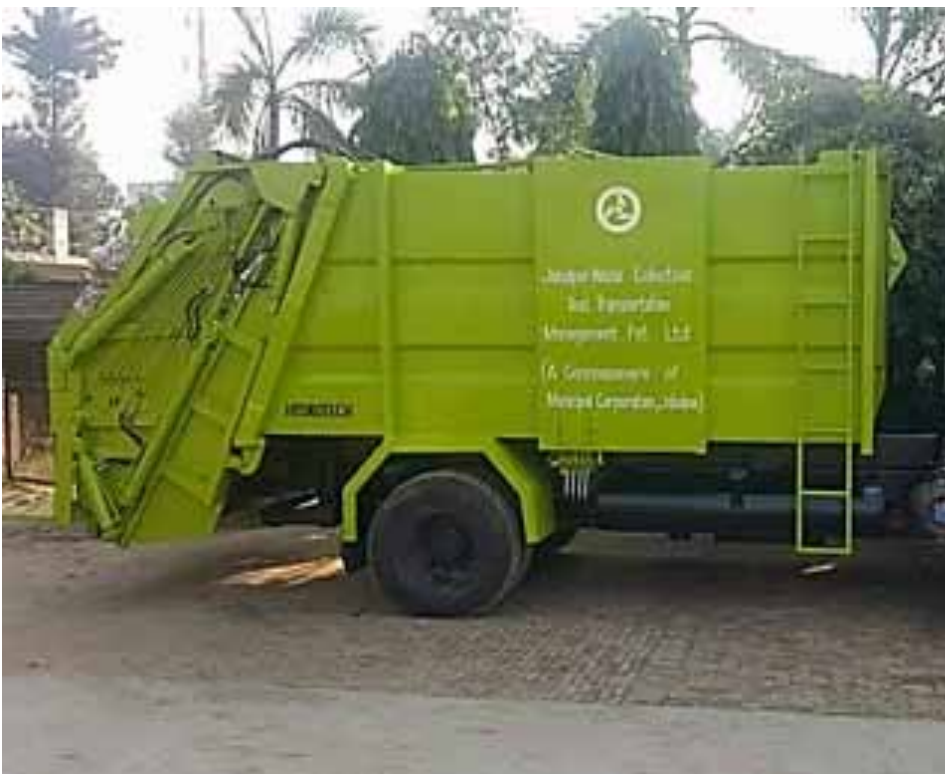
Deployed garbage collection and transportation vehicle
