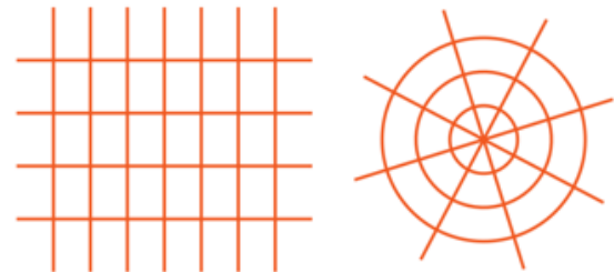
Figure 3 | Two types of Network Structures: Grid (left) Radial (Right) (Embarq (India), WRI (India), 2011)
