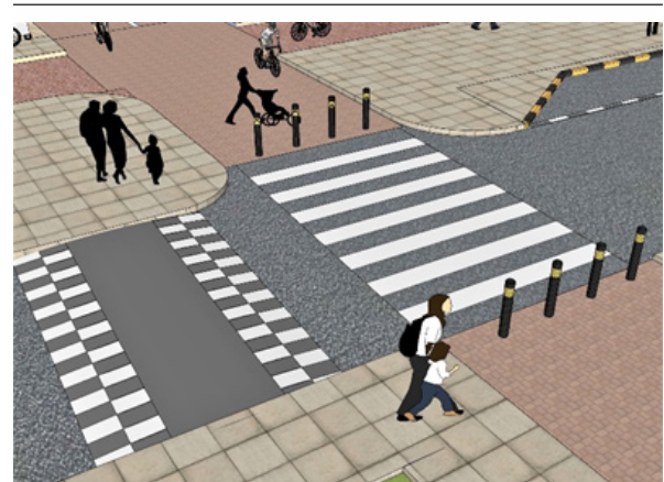
Figure 30 | Street infrastructure comprising of bollards, table top crossings and walkways
