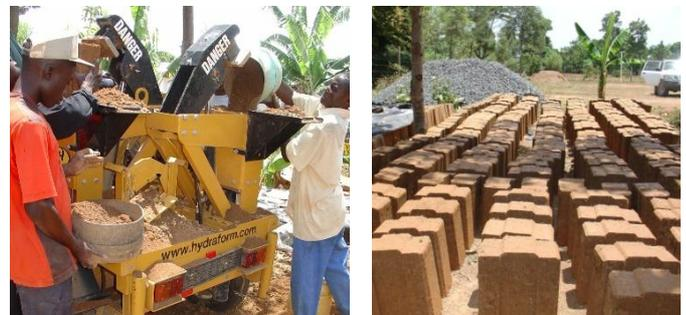
**Fig. 14:** Left: Production of hydraform blocks; Right: completed hydraform blocks (Source: Paul Mboya, June 2009).
