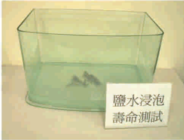
■ Salt Water Corrosion Test
