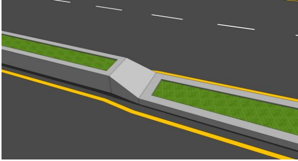
Figure 12 Retrofitting piece - cast in-situ RCC element to facilitate easy transition between old and new medians
