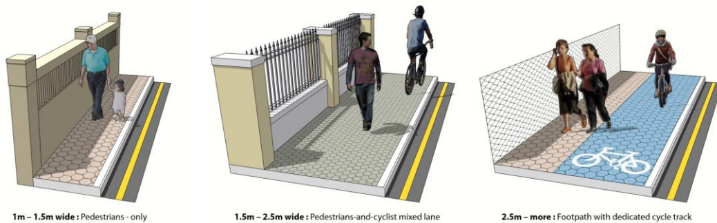
Figure 8 Types of proposed footpaths
