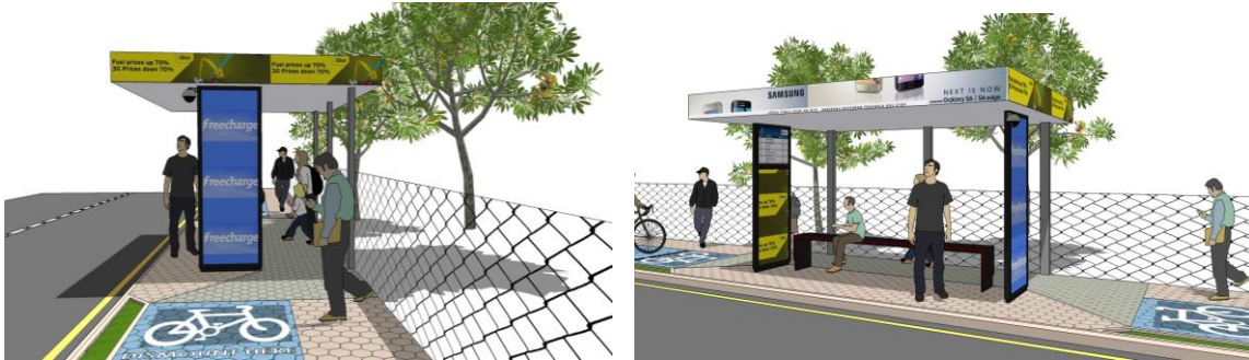
Figure 10 Bus Stop Type 1 (for footpaths more than 2.75m wide)
