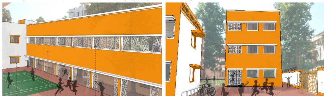
contrasting frames bright solid color facade jaalis for safety white band defining parapet projection with contrasting color school gate boundary wall with contrasting coping
