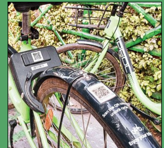
Fig 3. Cycle Locking System by QR Code
