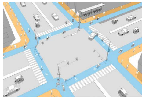
Figure 4.33: Segregated through cycle lanes at intersection
