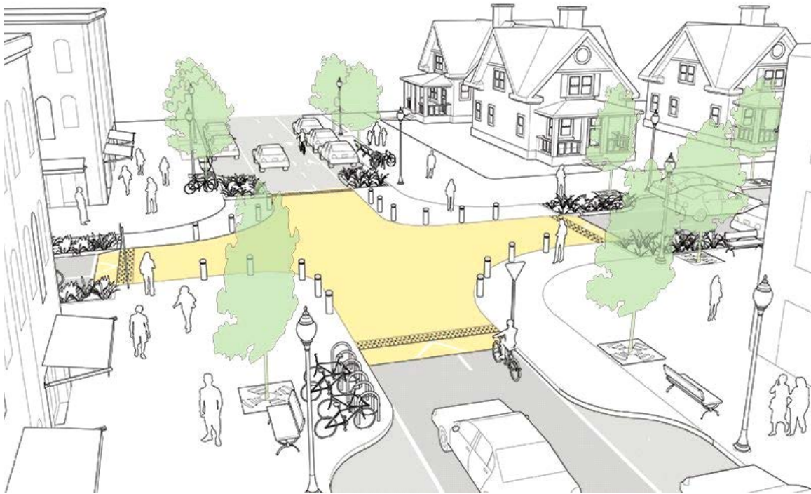
Figure 4.12: A raised intersection
